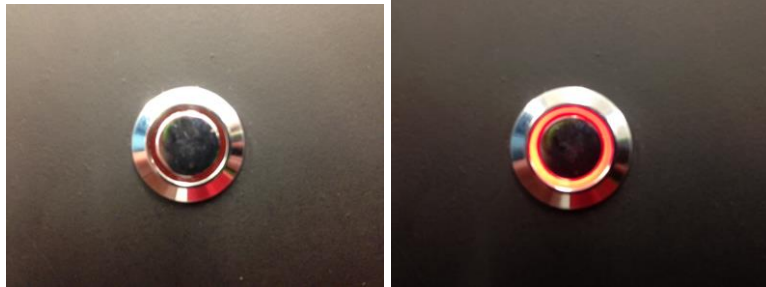
Figure 46: Discharge Capacitor button
