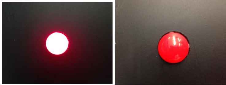
Figure 48: Capacitor Charged LED ON/OFF
